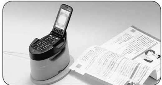
A document containing a Uni-Voice barcode and the device used to read it.
